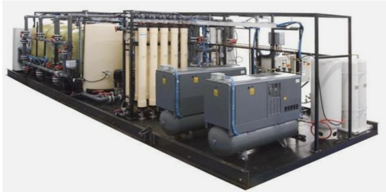
Figure 4. A modular unit of the DaguaFlo drinking water treatment plant
